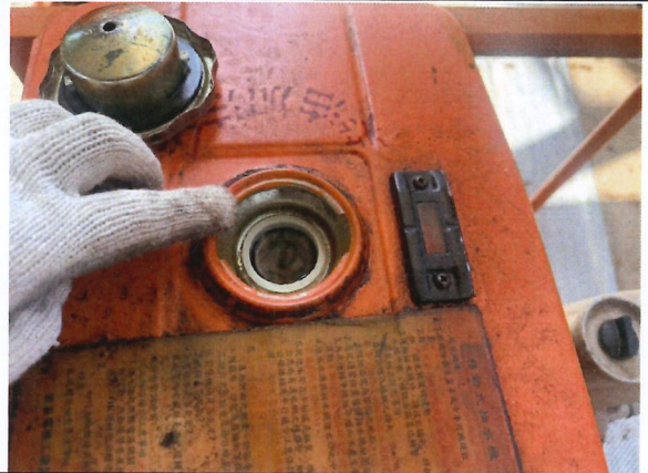
102-S007-02-燃油油位檢查
