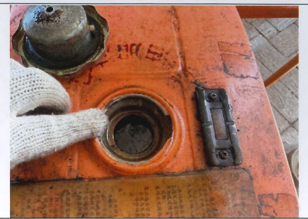
102-S009-02-燃油油位檢查
