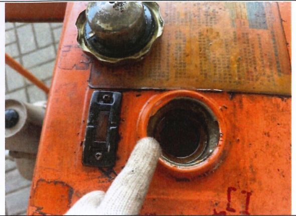
102-S009-02-燃油油位檢查
